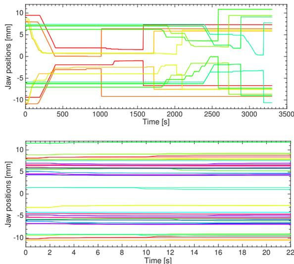
Figure 4: Time required to align the 8 TCTs in IR1 and IR5 in 2012 with the BLM-based technique (top) and all 16 TCTPs in 2015 with the BPM-based technique (bottom).
