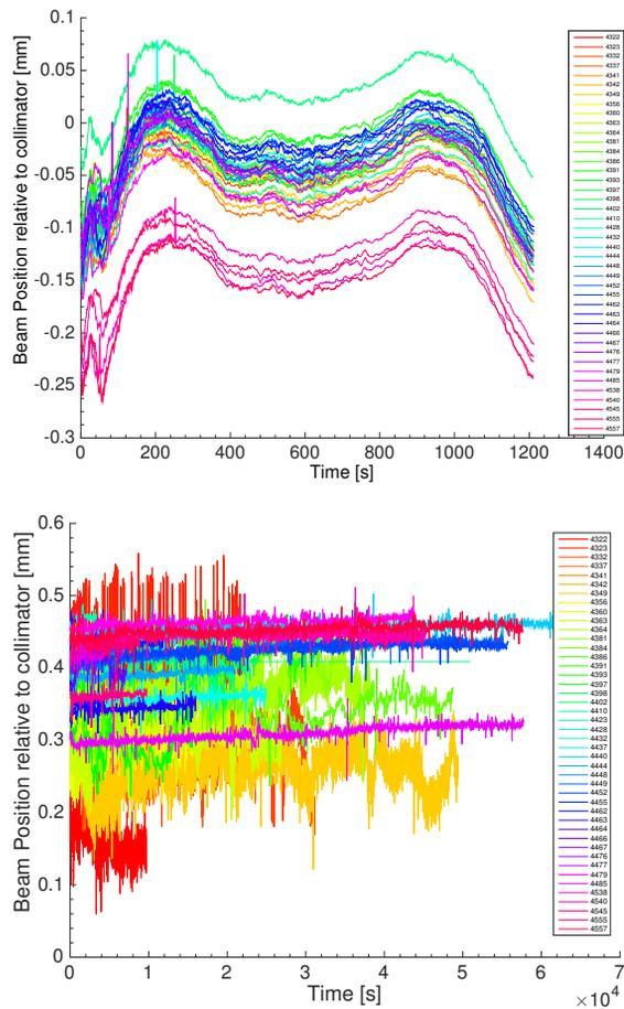
Figure 5: Beam positions measured relative to the centers of selected collimators during the ramp (top) and stable beams (bottom).
