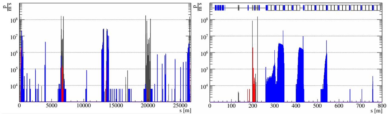
Figure 2: Expected beam loss pattern along the entire ring (left) and on the left side on IP1 (right) due to physics debris coming from IP1 and IP5, for  $\mathcal{L} = 7.5 \times 10^{34} \text{ cm}^{-2}\text{s}^{-1}$  and  $\sigma_{\text{inel}} = 81.2 \text{ mb}$  at 7 TeV.
