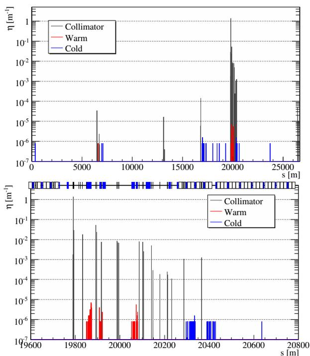
Figure 1: Expected beam loss pattern along the entire ring (top) and in IR7 (bottom) for an horizontal loss map. Blue: losses on cold magnets; Red: losses on warm magnets; Black: losses on collimators.
