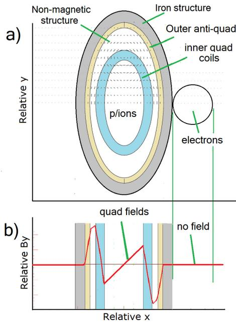
Figure 2: Elliptical quadrupole (blue) with outer cancelling anti-quadrupole (yellow), the grey area is an iron shield; a) cross section of coils with location of electron beam; b) vertical fields vs. horizontal position on the mid plane showing field cancellation.
