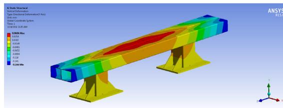
Figure 2: ANSYS result for thermal difference study.
