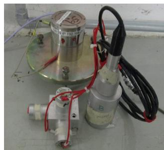
Figure 3: HLS, tri-axial geophone and seismometer.
