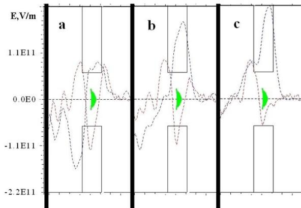
Figure 4: Longitudinal (red dash line) and transverse (blue dash line) plasma wave electric field distribution near the iris at radius 12 μm (a), 18 μm (b) and 24 μm (c). Iris radius 30 μm.
