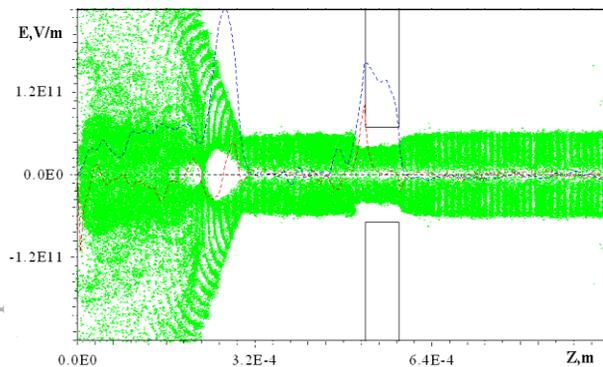
Figure 5: Plasmas electron component (green dots), longitudinal (red dash line) and transverse (blue dash line) plasma wave electric field distribution at the channel edge. Time moment 1000 fs after laser pulse started.
