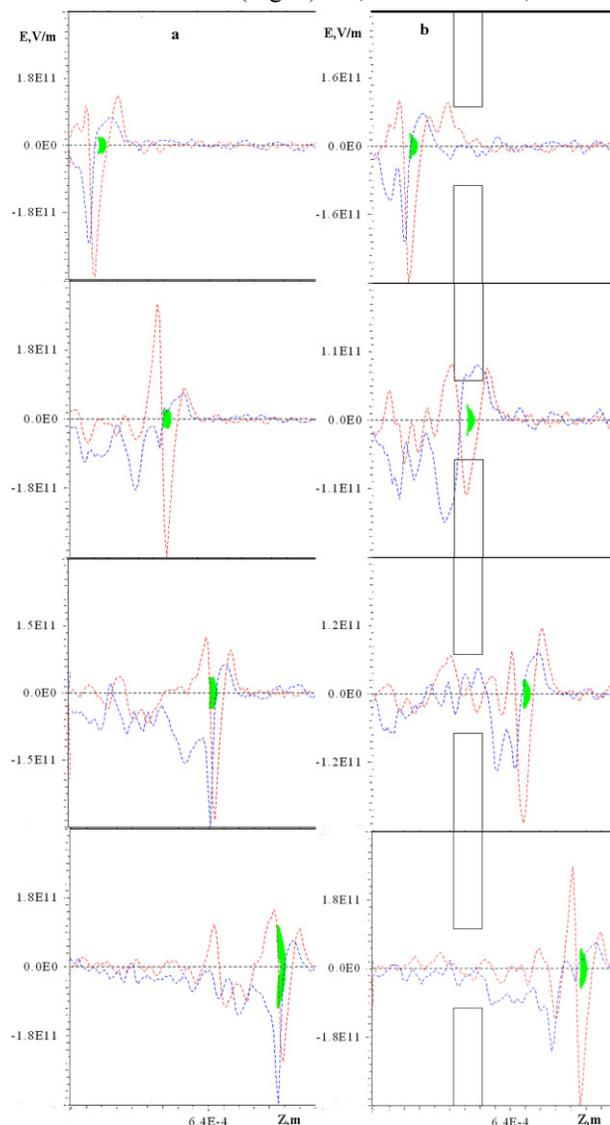
Figure 2: Time dependent (time step 400 fs) electron bunch (green dots), longitudinal (red dash line) and transverse (blue dash line) plasma wave electric field distribution in channel at the mean beam radius with (b) and without (a) iris.
