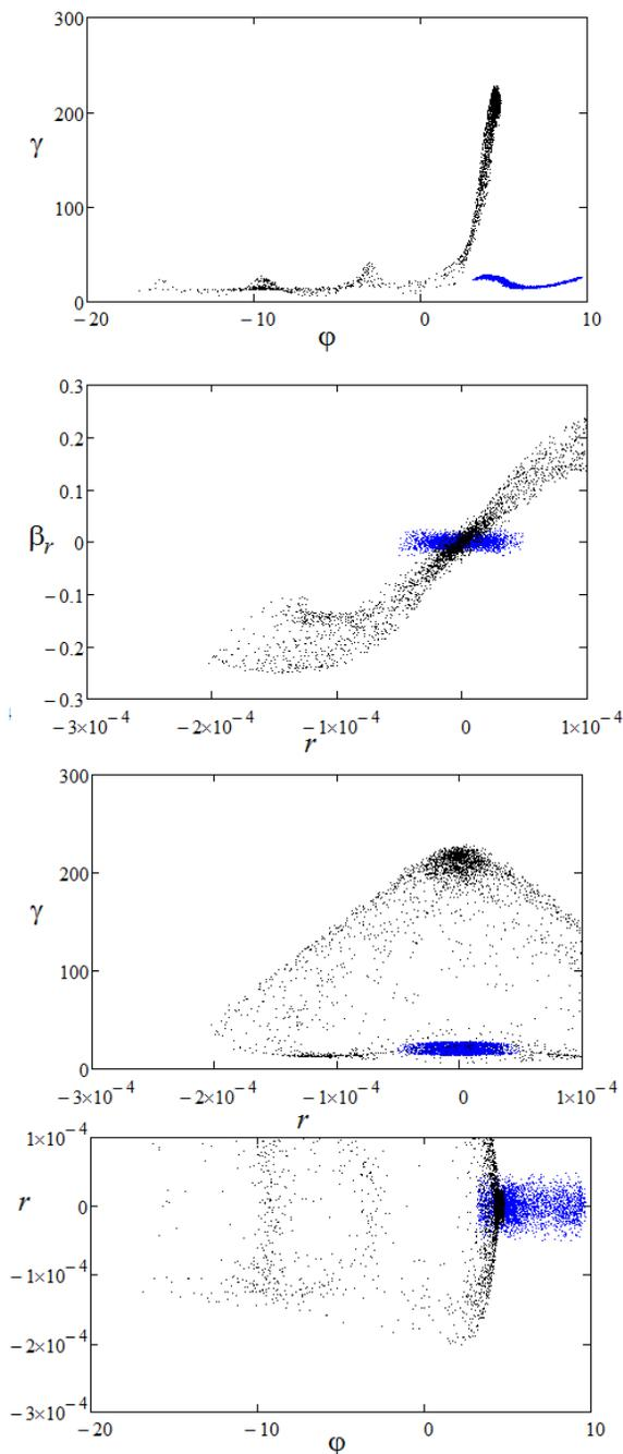
Figure 1: Results of 2D electrons dynamics simulation [3] for beam after pre-modulation for  $z=1000 \lambda_l$ ; are shown (top to bottom): particles distribution in conventional ( $\gamma$ ,  $\phi$ ) and ( $\beta_r$ ,  $r$  [m]) phase planes and in non-conventional ( $\gamma$ ,  $r$ ) and ( $r$ ,  $\phi$ ) planes, Injection distributions after pre-modulation are plotted by blue points and output by black.
