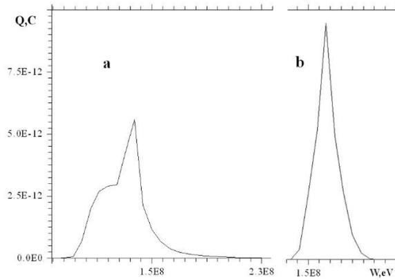
Figure 3: Electron bunch energy spectrum with (b) and without (a) iris.
