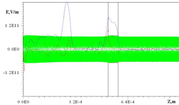
Figure 6: Plasmas ion component (green dots), longitudinal (red dash line) and transverse (blue dash line) plasma wave electric field distribution at the channel edge. Time moment 1000 fs after laser pulse started.
