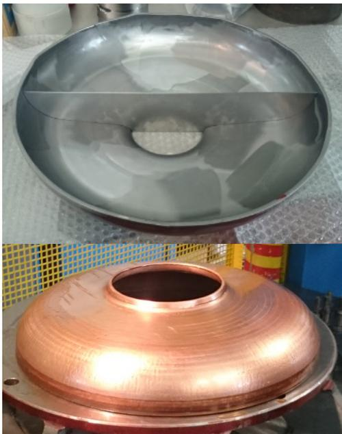
Figure 4: Deep drawing tests for INFN-LASA prototype cavities (up: inner Half Cell in LG Nb; down: end HC in Copper).
