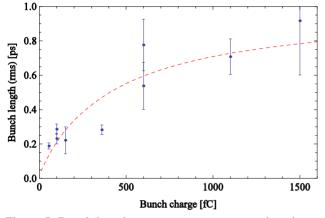
Figure 5: Bunch length measurements, compared to simulations (dotted line).
