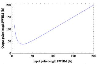
Figure 7: Laser pulse length after transport through  $2 \text{ mm CaF}_2$ .
