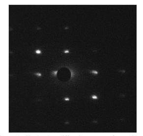
Figure 4: Single shot diffraction pattern from 100 nm thick Si(100).
