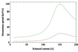
Figure 2: Simulated momentum spread at the sample as a function of solenoid current for a 1 pC beam (rms of distribution in red, full spread in green).
