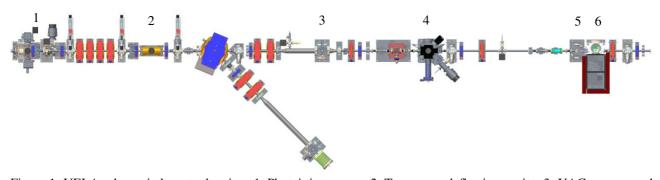
Figure 1: VELA schematic layout, showing: 1. Photoinjector gun, 2. Transverse deflecting cavity, 3. YAG screen used for bunch length measurements, 4. Sample chamber with independent stages for sample and beam shaping apertures, 5. Insertable Faraday cup, 6. Lanex screen used for imaging diffraction patterns.
