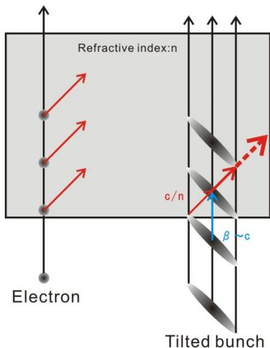
Figure 2: Cherenkov radiation from the tilted electron bunch.
