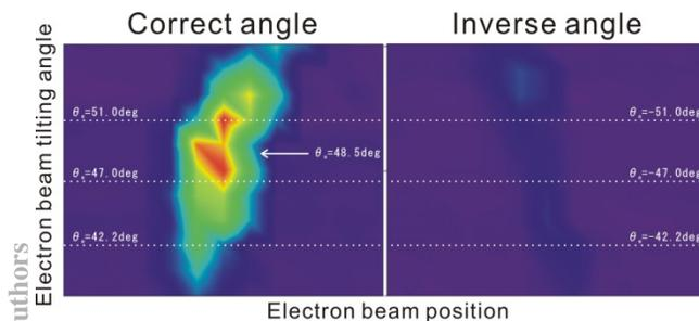
Figure 6: THz intensity as a function of the electron bunch position and electron bunch tilting angle.
