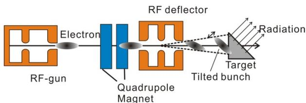
Figure 3: Experimental setup for coherent Cherenkov radiation by using tilted electron bunch.
