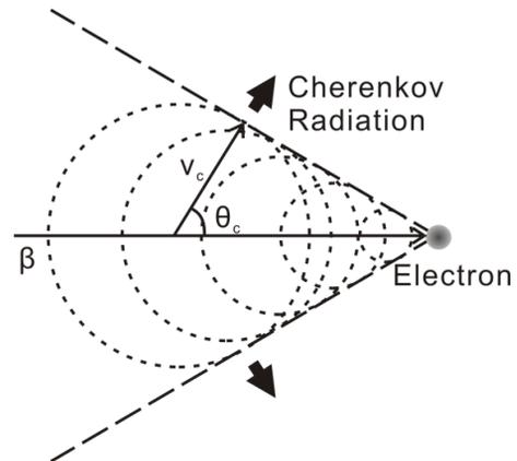
Figure 1: Schematic of Cherenkov radiation.
