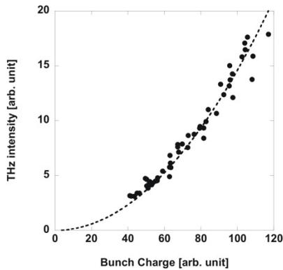
Figure 5: THz pulse intensity detected by QOD and 0.9 THz BPF as a function of the electron bunch charge.
