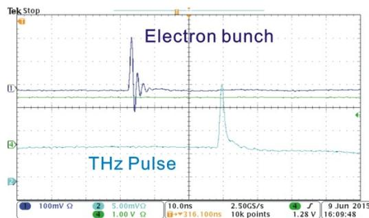
Figure 4: Electron beam signal detected by FCT (purple: top) and THz pulse signal by QOD detector (blue: bottom).
