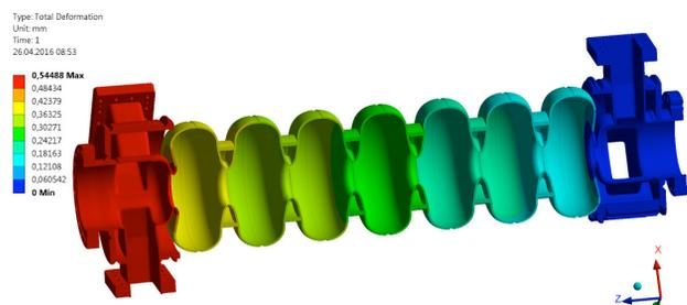
Fig. 7: Total deformation under 5 kN tuning force between the vessel flanges (right side fixed), computed with ANSYS [9] for 2 K Niobium of 3 mm wall thickness. Whereas the inner half cells are compressed by  $\sim 25 \mu\text{m}$ , both end half cells experience  $\sim 90 \mu\text{m}$ , the end-groups in total  $\sim 45 \mu\text{m}$ .
