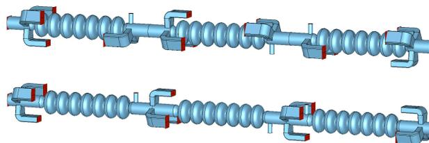
Fig. 1: Top: Baseline 3x5WG geometry, bottom: backup version 4x3WG with waveguide groups separated from the cavities. The fields at all waveguides, both beam pipe exits and the three coaxial FPCs (all marked in red) are evaluated in sets of the first 20 (50, 11 resp.) modes. This makes all the ports reflection-free terminated.
