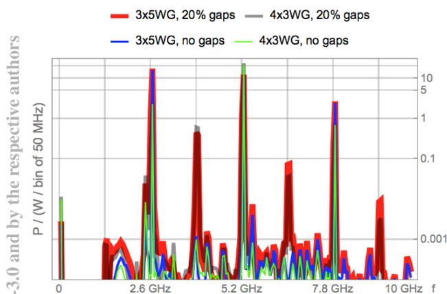
Fig. 5: Spectral resolved waveguide power, summed up over all waveguides. Relevant contributions only happen close to the beam harmonics (abscissa grid lines). The 2.6 GHz-line is more pronounced in the 3x5WG setup, whereas the 4x3WG setup has highest power levels at 5.2 GHz.
