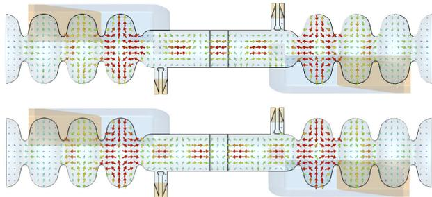
Fig. 3: Pair of beam-pipe-localised modes found in CSTMicrowaveStudio© [6] eigenmode simulations at (top) 2.4347 GHz with  $R/Q = 79.3 \Omega$ , (bottom) 2.4364 GHz,  $R/Q = 55.2 \Omega$ . The rotational symmetry of the  $TM_{01}$ -like field pattern in the beam pipe is distorted.
