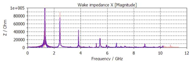
Fig. 2: Almost identical longitudinal beam impedance spectra (absolute value) of 3x5WG (light red) and 4x3WG (blue). The fundamental mode peak is clipped.
