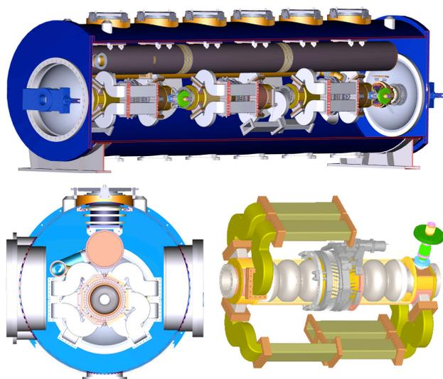
Fig. 6: Provisional layout of the bERLinPro Linac module seen from the side and the front together with the tank/waveguide arrangement of a single cavity. Straight waveguide sections will include the HOM absorbers.
