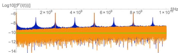
Figure 4: Lowest 10 GHz of the logarithmic-scaled current spectrum in relative units of the bERLinPro cw-beam. Orange: including jitter (cf. main text) and recirculation of the beam. Blue: also with 520 gaps after each 2080 bunches (96.25 pC bunch preserving total current of 100 mA). Green: Single bunch of 77 pC in 8  $\mu$ s.
