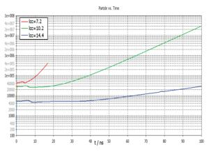
Figure 3: Plot of the temporal evolution of the number of particles due to SEE over 100 ns for several lengths of CC:  $l_{\text{CC}}$ = 7.2 mm (red), 10.2 mm (green) and 14.4 mm (blue) at  $E_{\rm acc}$ =1 MV/m. The red line stops at 17 ns, because MP was detected by the solver.
