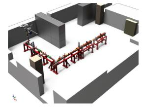
Figure 5: Test setup of STEAM, MELBA and MAMBO No. 1 & No. 2 in the MEX-3 hall. For a better overview the supports of STEAM are suppressed.
