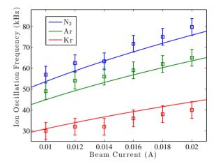
Figure 7: Resonance frequencies for various beam currents and ion species. The circles represent data points, while the lines indicate theoretical predictions [3].
