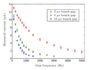
Figure 4: The number of trapped ions that reach the clearing electrode are reduced by increasing the frequency and duration of bunch gaps. The beam current was held fixed at 10 mA while taking this data.
