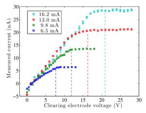
Figure 3: A picoammeter was used to measure the ion current striking the clearing electrode for different applied voltages. The vertical dotted lines mark the minimum voltage required for full ion clearing, as predicted using a simple model [3].
