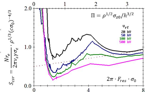
Figure 3: Thresholds for negative momentum compaction factor. The red dotted line is the simple scaling law found for  $\alpha > 0$ .
