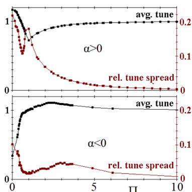
Figure 5: Average synchrotron tune and relative synchrotron tune spread for both signs of  $\alpha$  at the onset of the instability. For long bunches and large shielding factors both parameters are identical and the threshold should not depend on the sign of  $\alpha$ .
