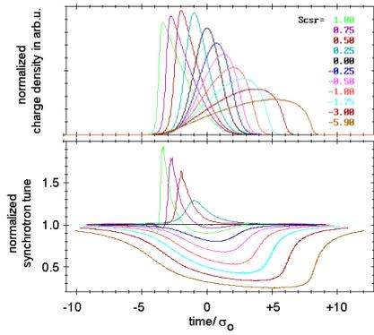
Figure 4: Result for very short bunches – without shielding of the CSR-interaction. Solutions of the Haissinski equation for the charge density and the normalized synchrotron tune derived from this distribution.
