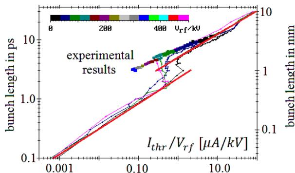
Figure 6: Comparison of experimental results measured by M. Ries at the MLS with the theoretical predictions. Approximations of the two solution branches are shown as red lines. The experimental results are shown as coloured squares with colours corresponding to the RF-voltage during the measurement.
