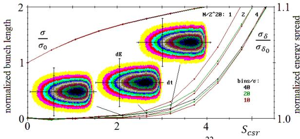
Figure 1: Results of tracking up to  $2^{22}$  particles with a bunch length of 2 ps. The number of bins per  $\sigma_0$  has only a small effect.
