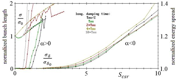
Figure 2: Comparison of multi particle tracking results for positive and negative compaction factors without shielding. In the calculation  $2^{22}$  particles and 20 bins/ $\sigma_0$  were used.
