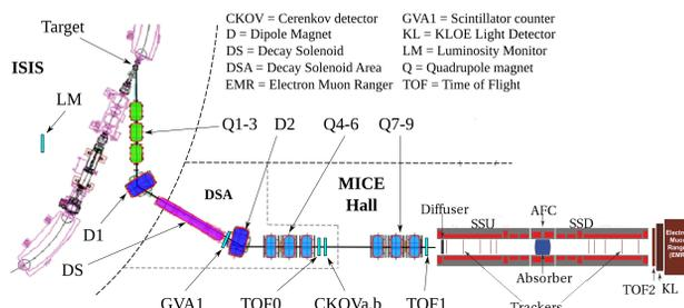
Figure 2: Plan view of MICE Step IV configuration, beginning from the target in ISIS.
