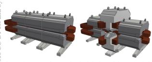
Figure 6: Perspective mechanical design of the main (left) and HFI (right) dipole magnets [7].
