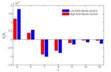
Figure 4: Normalized multipole errors at +14 mm in high and low field sections.
