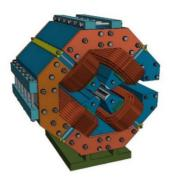
Figure 10: Perspective mechanical design of the SR quadrupole [7].
