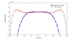
Figure 9: Integrated field quality of the quadrupole before and after chamfering.
