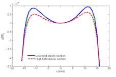
Figure 3: Field quality of the 2D designed high and low-field dipole sections within  $\pm 14$  mm GFR.
