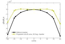
Figure 5: Integrated field quality of the HFI dipole magnet in the y=0 plane with and without chamfer. [8]
