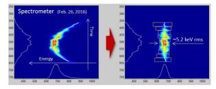
Figure 4: Example of a longitudinal phase space measurement for a 22 pC, 3.2 A peak current and 15.7 MeV beam. Left: full phase space. Right: phase space after removal of  $1^{st}$  and  $2^{nd}$  order correlations.
