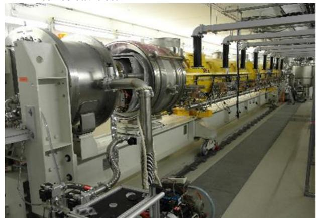
Figure 5: Cryomodule test-stand installation at AMTF.
