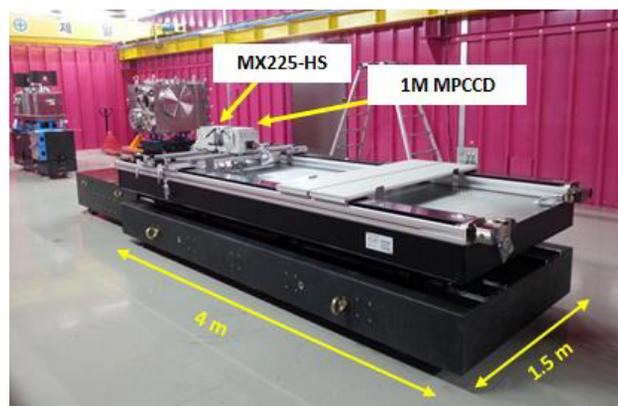
Figure 7: HES-2 detector stage. 1M MPCCD (for CXI) and MX225-HS (for SFX) will be installed in the arrow indicator.
