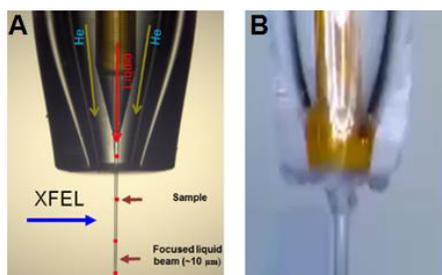
Figure 5: SFX sample delivery system. (A) liquid jet sample injector (B) LCP injector.
