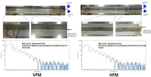
Figure 2: Carbon coated mirror substrate. VFM (vertical focusing mirror) and HFM (horizontal focusing mirror).
