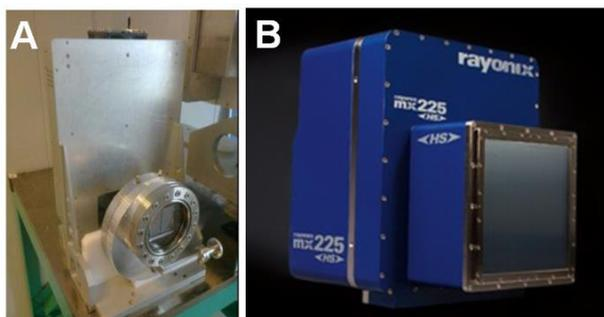
Figure 6: HES-2 detector systems. (A) 1M MPCCD (B) MX225-HS.
