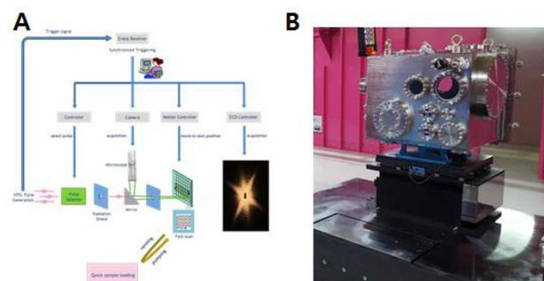
Figure 4: CXI sample chamber. (A) Schematic of sample-providing method. (B) CXI sample chamber.
