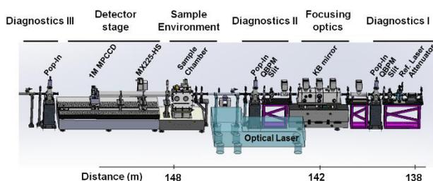
Figure 1. Overview of the HES2 experimental hutch. HES-2 instruments consist of the diagnostics, focusing optics, sample environment and detectors.
