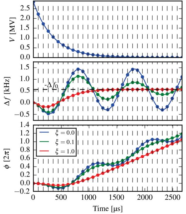
Figure 2: Voltage, RF frequency shift, and phase shift as in Fig. 1. The parameter  $\xi$  is varied, while  $f_m = 1$  kHz,  $\tau = 4$  turns = 356  $\mu\text{s}$  and  $V_0 = 2.85$  MV. Note that the vertical scale for  $\Delta f$  and  $\phi$  is not the same as in Fig. 1.
