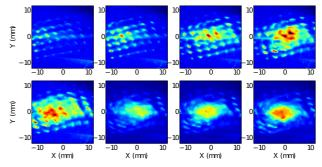
Figure 7: False color 50 MeV electron beam patterns for various charges. From left to right and top to bottom: Q=60pC, 100pC, 200pC, 300pC, 400pC, 500pC, 600pC, 700pC.
