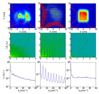
Figure 3: Measured UV laser without MLA (left column) and with MLA setup to produce beamlets (middle column) or as a homogenizer (right column). The upper, middle, and lower rows respectively correspond to the laser transverse density distribution, its 2D FFT, and the projected spectrum along the horizontal frequency  $k_x$ .
