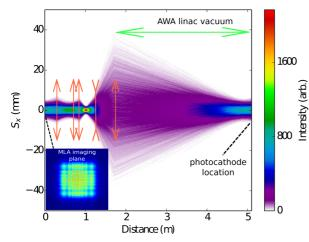
Figure 2: Ray tracing of a five-lens transport capable of imaging the homogenized beam to the photocathode (this system was built at AWA). The inset shows of a  $8 \times 8$  simulated through the MLA using srw [6] (bottom left).
