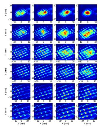
Figure 6: False color 8 MeV electron beam patterns for various matching solenoid current setting and charge. Left to right: Q=60pC, 80pC, 100pC, 120pC. Top to bottom: M=215A, 230A, 241A, 255A, 270A, 290A and BF=498A.
