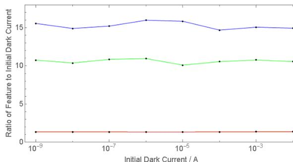
Figure 7: Ratios between the amplitude of the ghost pulse for a filled (blue) and empty (green) RF bucket, and the dark current plateau around the photoemitted bunch for both RF buckets (red), compared to the initial level of dark current. Measured at 3 m from the photocathode.
