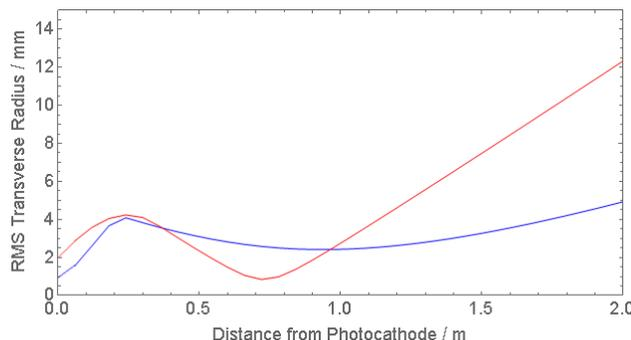
Figure 1: RMS transverse radius of photoemitted bunch (blue) and dark current (red) along the beam line.
