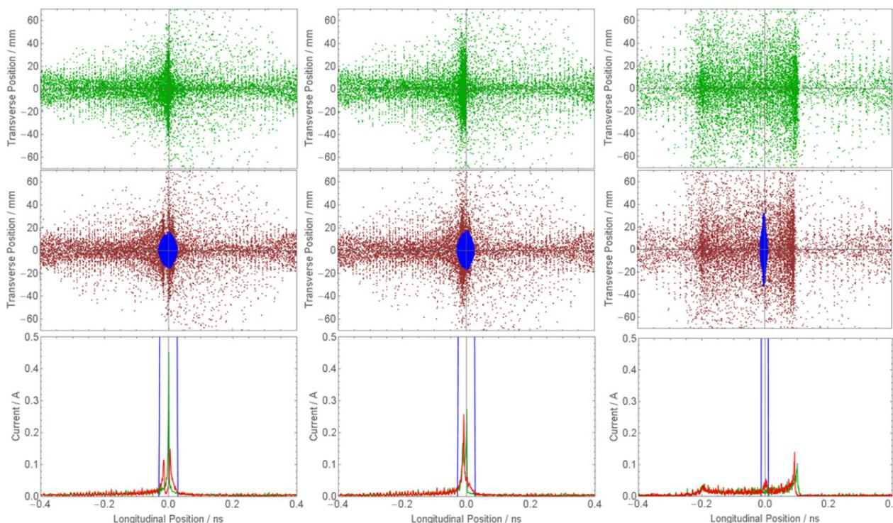
Figure 6: Particle distributions for an empty (top) and filled (middle) RF bucket and current profiles (bottom) with 10 mA dark current, at positions: from left to right; 1.98 m – maximal compression of dark current in empty RF bucket, 2.07 m – maximal compression of dark current in filled RF bucket and 3 m – maximal compression of photoemitted bunch. The photoemitted bunch (blue), dark current (red) and dark current in the empty RF bucket (green) are shown.
