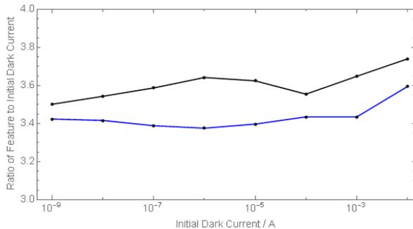
Figure 4: Ratio between the front (blue) and back (black) peaks in dark current and the initial level of dark current, results were taken at 3 m from the photocathode.
