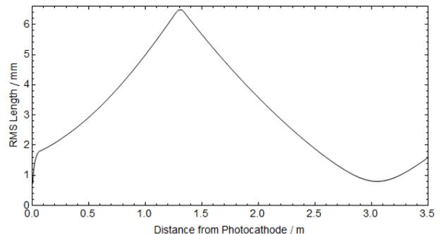
Figure 5: RMS length of photoemitted bunch.
