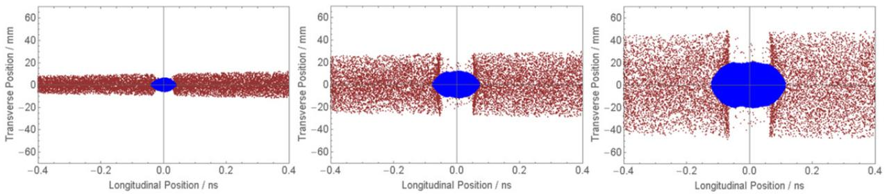
Figure 2: Longitudinal particle distribution for the simulation with 10 mA dark current, shown at different positions in the beam line. From left to right: 1.2 m, 2.07 m and 3.0 m from the photocathode. The macroparticles for the photoemitted bunch (blue) and dark current (red) are shown.
