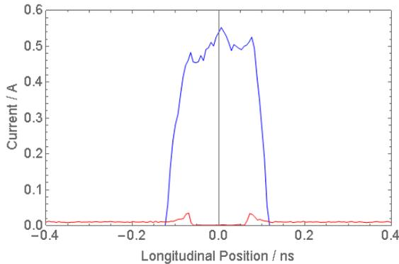
Figure 3: Current profile of photoemitted bunch with 10 mA dark current at 3 m from the cathode, the dark current (red), the photoemitted bunch (blue) are shown.
