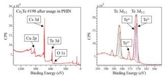
Figure 7: XPS spectrum (wide range and Te region) of cathode #198 after usage in PHIN 2014 [8].
