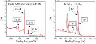
Figure 6: XPS spectrum (wide range and Te region) of cathode #203 after usage in PHIN 2015 [8].
