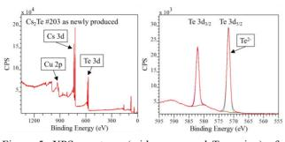
Figure 5: XPS spectrum (wide range and Te region) of cathode #203 as newly produced [8].
