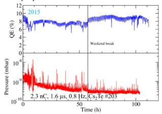
Figure 3: Lifetime measurement of  $Cs_2Te$  cathode #203 with 2.3 nC/bunch, 1.6  $\mu s$  train length and 0.8 Hz macropulse repetition rate.
