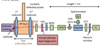
Figure 2: Layout of PHIN. Fast current transformers (FCT), vacuum mirror (VM), steering magnet (SM), beam position monitor (BPM), multi-slit mask (MSM), optical transition radiation screens (OTR), gated cameras (MTV), segmented beam dump (SD), Faraday cup (FC).
