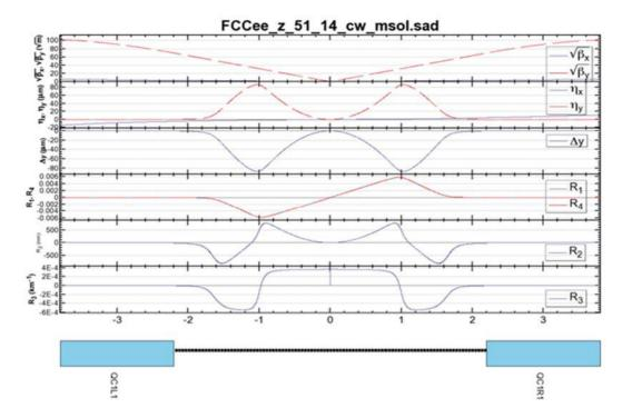
Figure 4: Beam optical functions between the centers of the final quadrupoles of the proposed solution. Columns are, from top to bottom,  $\sqrt{\beta_x}$  and  $\sqrt{\beta_y}$ , x and y dispersion, y orbit,  $R_1$  and  $R_4$ ,  $R_2$ ,  $R_3$ , where  $R_{1,2,3,4}$  are the x-y coupling parameters. The vertical orbit, dispersion, and the coupling parameters are confined within the compensation solenoid.
