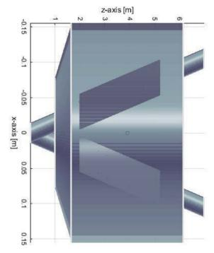
Figure 1: The conceptual design of the magnetic elements close to the IP, looking on the x-z plane. The IP is at (0,0). Please note the elongated scale in x. The opening angle of the (schematic) beam pipes is 30 mrad. The final focus quadrupoles surround the two beam pipes whereas the rest of the elements are aligned to the longitudinal axis of the experiment. The compensating solenoid is tapered and is in front of the screening solenoid. The detector solenoid is outside this picture.
