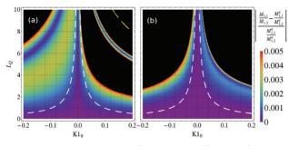
Figure 2: The absolute value of the relative difference of the ratio  $M_{1,1}/M_{2,1}$  from the ratio  $M_{1,1}^q/M_{2,1}^q$  as a function of different  $K1_0$  and  $L_Q$ , for the TEAPOT<sub>5</sub> (a) and the CSABA<sub>2</sub> (b). The area between the white dashed lines guarantees stable motion through a symmetric FODO cell.
