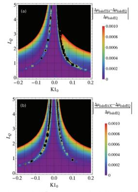
Figure 3: Using the different integrators, the absolute value of the relative difference of  $\Delta \mu$  from  $\Delta \mu_{fodofEQ}$  is calculated, for the TEAPOT<sub>4</sub> (a) and the CSABA<sub>3</sub> (b).
