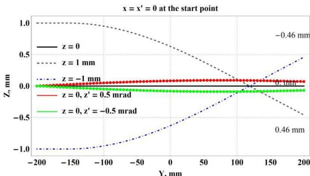
Figure 3: The electron trajectory in vertical plane with different start point  $z = -1, 0$  and  $1$  mm (curves) and  $z' = \pm 0.5$  mrad (dots).
