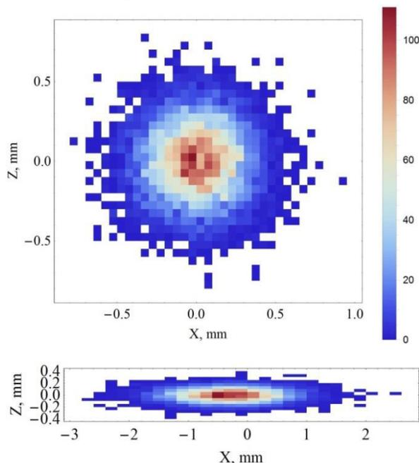
Figure 4: Example of random gaussian electron transversal distribution at start point (up,  $Y = -200$  mm) and at end point (bottom,  $Y = 200$  mm) with  $10^4$  particles. Both horizontal and vertical sizes are equal to  $0.2$  mm (rms) for upper picture. The legend is the same for both pictures.
