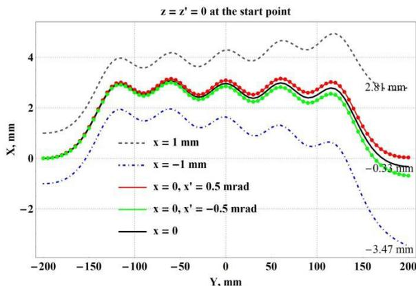
Figure 2: The electron trajectory in horizontal plane with different start point  $x = -1, 0$  and  $1$  mm (curves) and  $x' = \pm 0.5$  mrad (dots).
