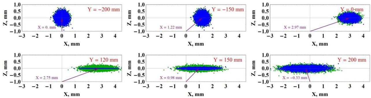
Figure 5: Transversal beam profile evolution along Y axis without divergence (blue central dots) and with divergence (green halo dots), where -150 and 150 mm are wiggler magnet edge, 120 mm is the maximum vertical focusing (see Fig. 3), -200 and 200 mm are the locations 50 mm far from both magnet edges.
