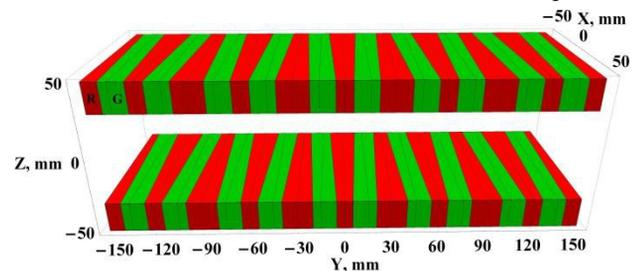
Figure 1: 3D wiggler model with 60-mm gap, where X is the horizontal axis and Z is the vertical axis, Y is the longitudinal axis. The origin is the center of the wiggler. Red (R) and green (G) blocks have a vertical and horizontal magnetization respectively.
