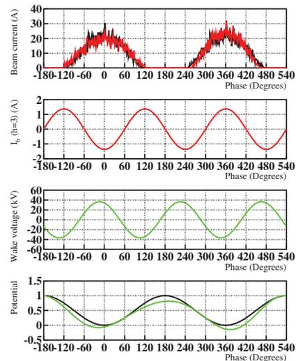
Figure 3: Bunch shape, beam current, wake voltage of  $h = 3$  and potential well of the fundamental rf and the wake voltage of  $h = 3$  arisen from the bunch deformation where the first bunch becomes wider and the second bunch becomes narrower.
