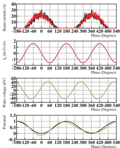
Figure 5: Bunch shape, beam current, wake voltage of  $h = 3$  and potential well of the fundamental rf and the wake voltage of  $h = 3$  arisen from the bunch displacement where the bunches move apart from each other.
