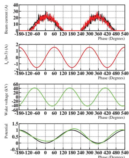
Figure 4: Bunch shape, beam current, wake voltage of  $h = 3$  and potential well of the fundamental rf and the wake voltage of  $h = 3$  arisen from the bunch displacement where the bunches get closer to each other.
