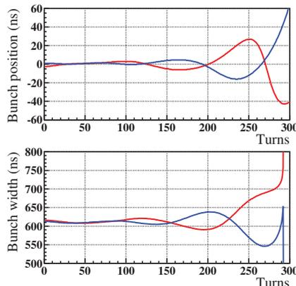
Figure 6: Simulation result of the bunch position and the bunch width under the beam loading of  $h = 3$ .
