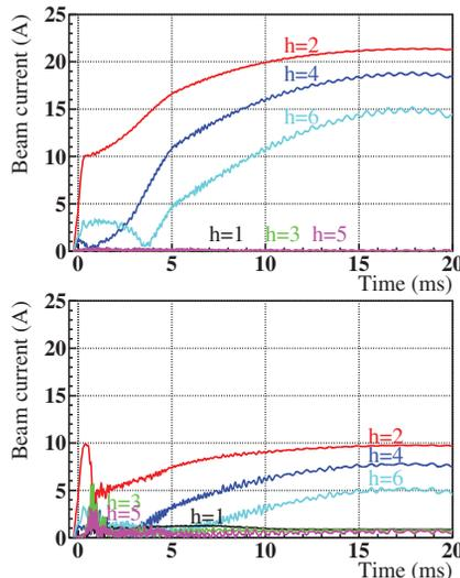
Figure 1: Simulation result for each harmonic of the beam current during the acceleration. The upper graph is the case without the beam loading and the lower graph is the case with the beam loading. The even harmonics of the beam loading are compensated.
