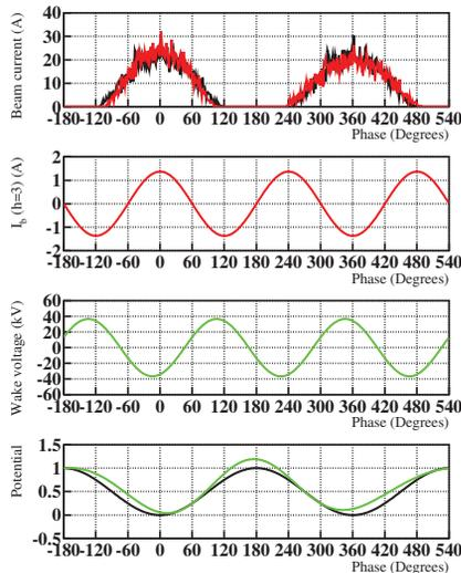
Figure 2: Bunch shape, beam current, wake voltage of  $h = 3$  and potential well of the fundamental rf and the wake voltage of  $h = 3$  arisen from the bunch deformation where the first bunch becomes narrower and the second bunch becomes wider.
