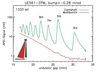
Figure 4: Gated X-ray APD signal recorded during a gap scan of the UE56-Apple II undulator at shift 25 (elliptical mode). The island orbit was aligned to the undulator and beamline axis while the standard orbit passes far off-axis blocked by apertures (insert). Light from the island (green) shows harmonics and from the core beam (red) does not.
