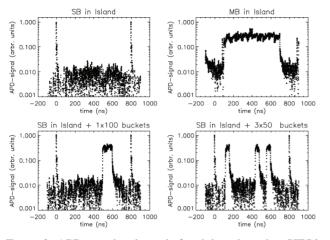
Figure 3: APD signal at the end of undulator beamline UE56 if island orbit adjusted on undulator axis. Different fill patterns have been stored on the island orbit.
