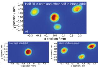
Figure 2: Source point image taken by a hard X-ray pinhole camera (8 keV) at a regular ring dipole at a  $3^{rd}$  order resonance. a) Half of fill in core and other half in islands, b) all current in core and c) all current in island orbit.
