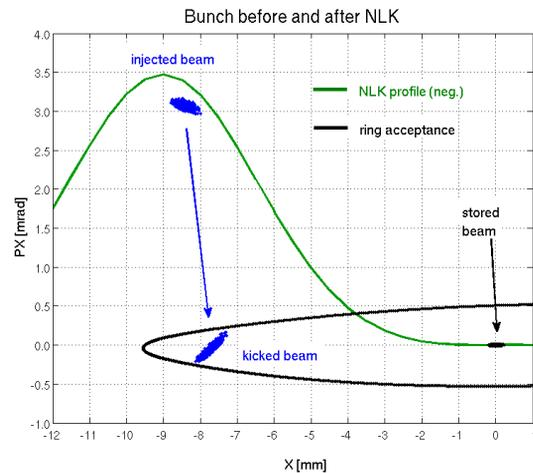
Figure 4: Phase space around the NLK position. Blue dots are 1000 particles representing the injected beam before and after the nonlinear kick. Green curve represents the negative of the NLK profile. Black dots correspond to the stored beam at  $x=0$  mm and the ellipse is the nonlinear acceptance of the storage ring defined by an average dynamical aperture of 9.5 mm in the horizontal plane calculated from 20 simulated machines with realistic random errors.
