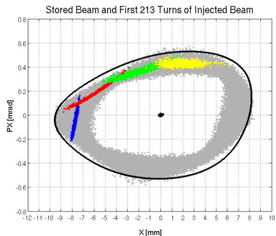
Figure 5: Phase space right pass the NLK with tracking data of the injected beam. In blue, 1000 particles representing the injected beam right after the nonlinear kick. In red, green and yellow, the injected beam after one, two and three turns around the storage ring, respectively. Depicted in grey is the beam in the next 210 turns.
