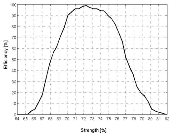
Figure 6: Injection efficiency as a function of the NLK strength calculated by particle tracking.
