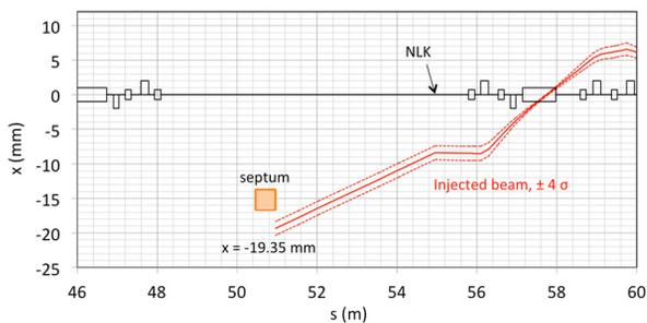
Figure 3: Injection into the storage ring using a NLK. The trajectory of the injected beam centroid in the horizontal plane is shown in solid red curve. The dashed curves represent  $\pm 4\sigma_x$  beam envelope.
