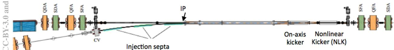
Figure 1: Layout of the Sirius storage ring injection straight section. The on-axis injection kicker and the nonlinear kicker are located downstream the injection point (IP), in the same straight section.
