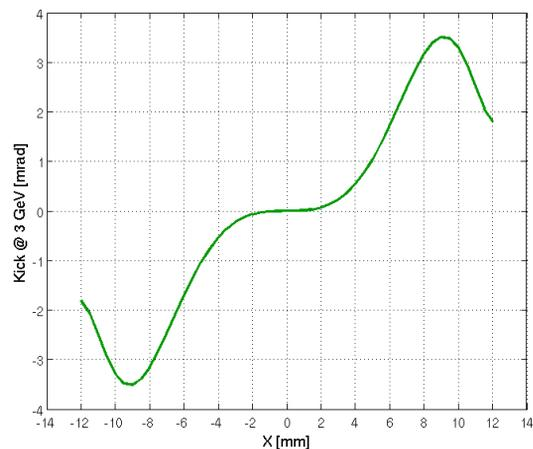
Figure 7: Calculated nonlinear kick profile. A peak kick of 4.8 mrad is obtained at around  $x=-9$  mm. This kick corresponds to a field of 107 mT for the 0.45 m-long kicker model excited with a current of 1850 A.
