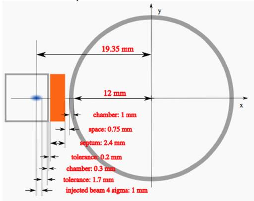
Figure 2: Schematic representation of the transverse cross section at the storage ring injection point.
