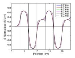
Figure 3: Longitudinal fields at subsequent radii cross the bore tube and first six cells.
