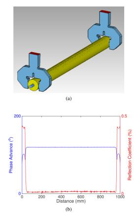
Figure 1: a) A CST drawing of the 30 cell linac with couplers. b) Evolution of phase advance and the reflection coefficient along the linac.
