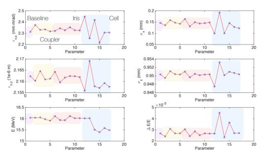
Figure 7: Various beam dynamics observables as a function of geometric modifications on the linac cells.
