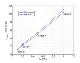
Figure 6: Beam emittance as a function of the charge per bunch.
