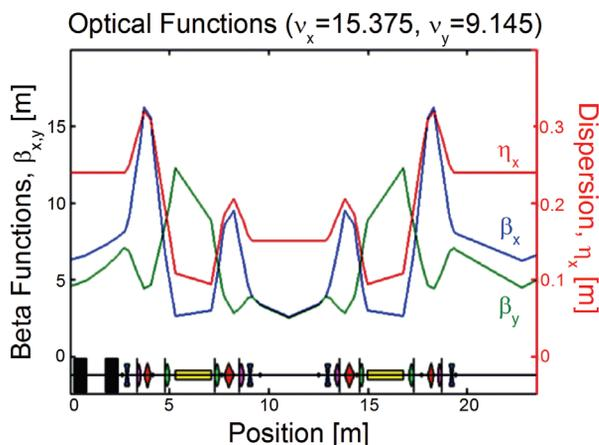
Figure 1: PLS-II lattice function of a half cell.
