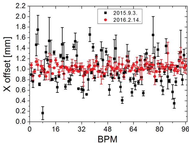
Figure 5: Beam-based alignment in horizontal plane. BPM's center set as 1 mm out of the quadrupole center.
