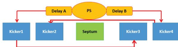
Figure 2: The injection system consists of a Lambertson septum and four kicker magnets. There are two timing-delay units and one strength knob.
