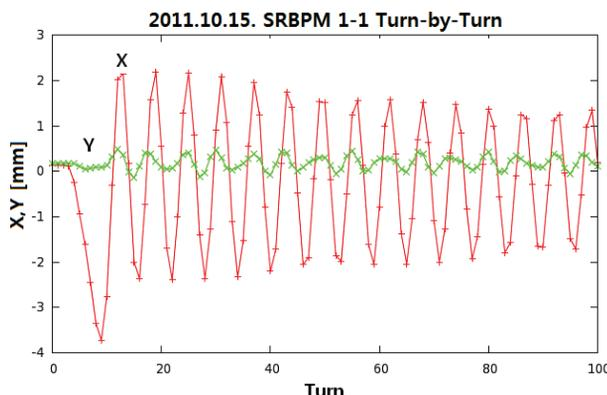
Figure 3: An example of the injection bump leakage at the first BPM in the commissioning.
