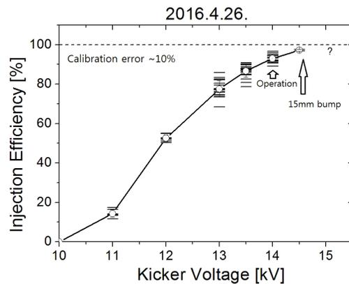
Figure 7: The injection efficiency as a function of the kicker strength.
