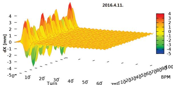
Figure 4: The injection bump leakage in horizontal plane after tuning.
