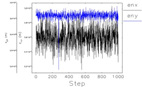
Figure 10: The normalized emittance of MID-FEL after correction.
