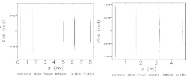
Figure 8: The correctors strength (left: MID right: FAR). As can be seen in Fig. 8. For FAR-FEL, the maximum strength of correctors is lower than 1mrad. In the case of MID-FEL, the maximum strength of correctors is
