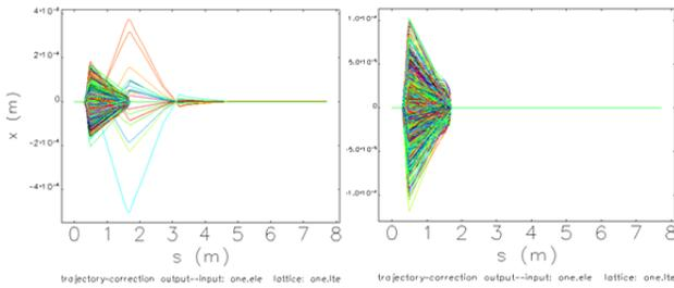
Figure 6: 1000 random seeds simulation of trajectory corrections of FAR-FEL transport line.
