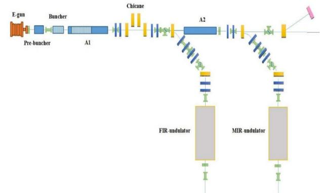
Figure 1: Basic layout of the FEL facility.
