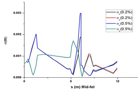
Figure 5: The beam envelope of different energy spread in MID-FEL transport line.
