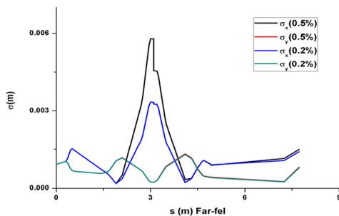
Figure 3: The beam envelope of different energy spread in FAR-FEL transport line.
