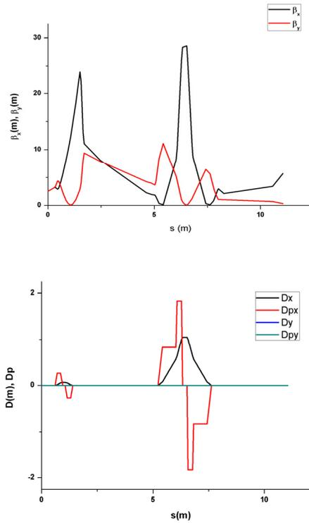
Figure 4: The optics of MID-FEL transport line.
