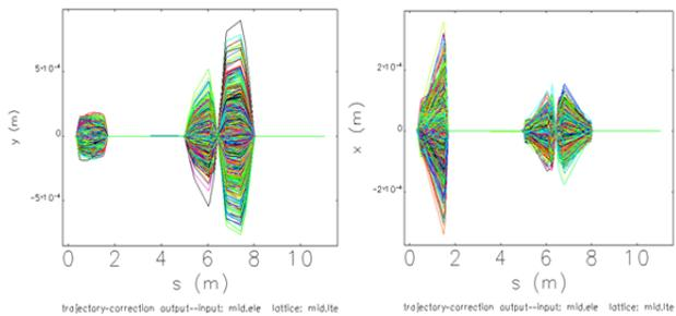
Figure 7: 1000 random seeds simulation of trajectory corrections of MID-FEL transport line.
