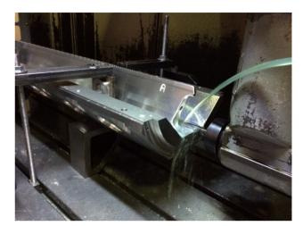
Figure 1: Machining of the cut-backs.
