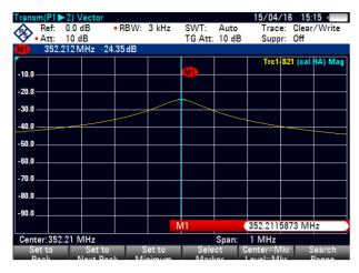
Figure 5: S21 curve from the resonant frequency tuning of the RFQ.
