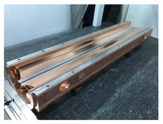
Figure 4: Assembling of the vanes.
