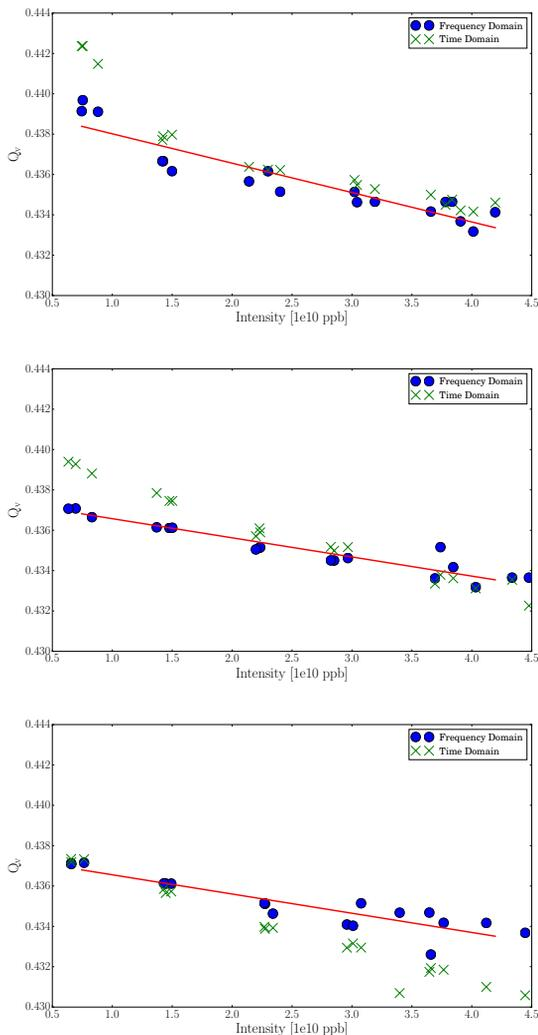
Figure 1: Vertical coherent tune shift as function of intensity for 10 (top), 20 (middle) and 30 (bottom) bunches using both the time domain and frequency domain methods. A linear fit of the frequency domain fit is also shown.
