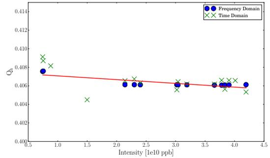
Figure 2: Horizontal coherent tune shift as function of intensity for 10 bunches using both the time domain and frequency domain methods. A linear fit of the frequency domain fit is also shown..
