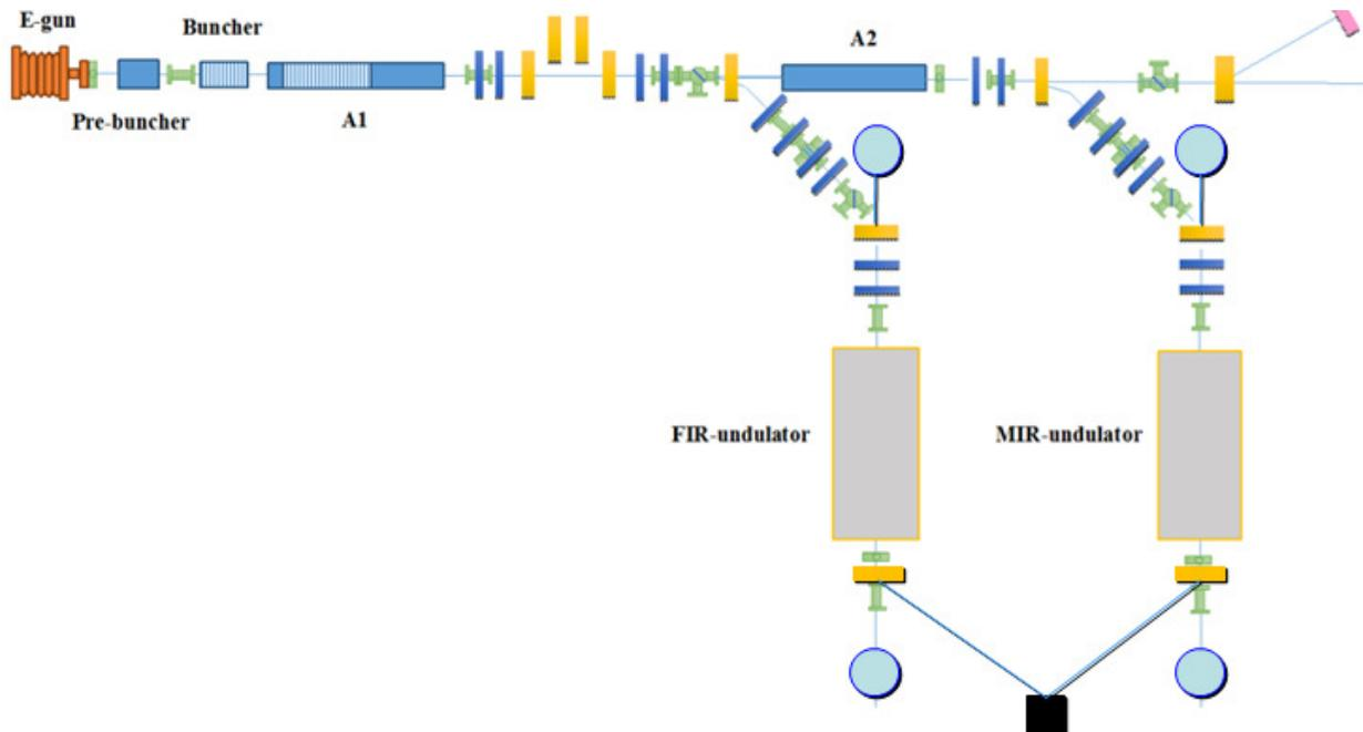
Figure 1: Schematic layout of the FELiChEM.
