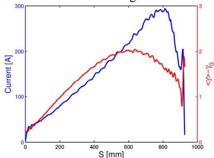
Figure 3: Beam current and energy distribution along the electron beam coordinate.
