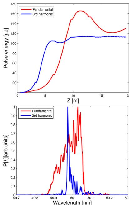
Figure 4: Comparison of 50 nm radiation of DCLS, the saturation length of harmonic lasing is about 5 m, while the fundamental is still in exponential gain regime.
