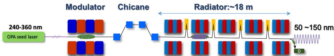
Figure 1: The schematic layout of harmonic lasing scheme in DCLS.
