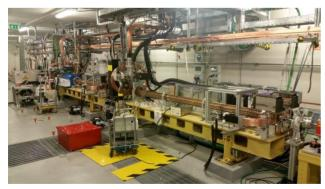
Figure 1: The new accelerating structures in the injector.
