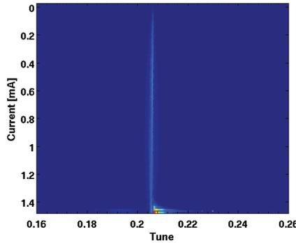
Figure 2: Horizontal measured betatron tune shift with current for  $Q'_x = 0, Q'_y = 3$  and  $V_{RF} = 2.5$  MV. The measured TMCI threshold is 1.47 mA.
