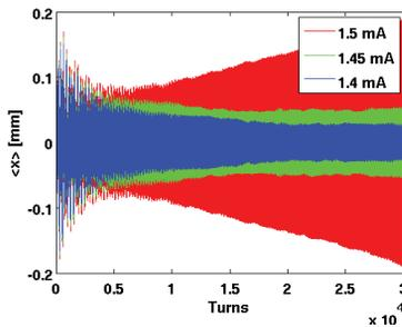
Figure 3: Horizontal centroid position over 30000 turns for single bunch current of 1.4, 1.45 and 1.5 mA. A growth in the centroid amplitude can be observed after 1.45 mA.
