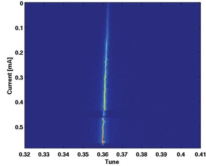
Figure 4: Vertical measured tune shift with current for  $Q'_x = 3, Q'_y = 0, V_{RF} = 2.5$  MV and closed IDs. The measured TMCI threshold is 0.6 mA.
