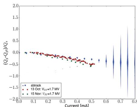
Figure 7: Vertical normalized betatron tune shift with current for  $V_{RF} = 1.7$  MV. The simulation (in blue) predicts a coupling of  $m = 0$  with a higher order head-tail mode  $m = -1$  at around 0.55-0.6 mA. The measured threshold is at around 0.51 mA.
