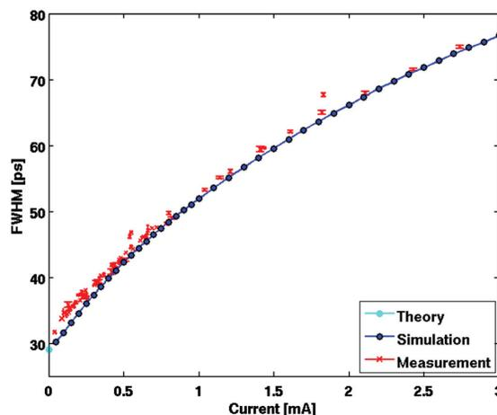
Figure 1: Bunch lengthening as a function of current. The measured data are shown in red and the sbrack simulation in blue. The longitudinal model impedance consists of RW, a BBR and an inductive impedance.
