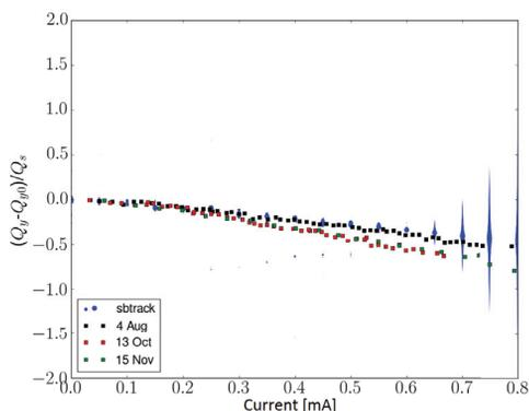
Figure 6: Vertical normalized betatron tune shift with current for open IDs. The simulation (in blue) predicts a coupling of  $m = 0$  with a higher order head-tail mode  $m = -1$  at around 0.7 mA. The measured threshold is at 0.74 mA.
