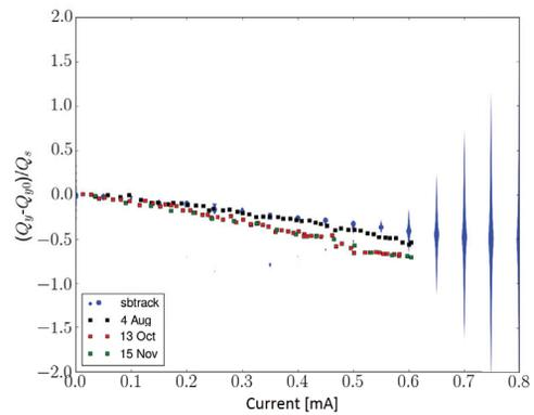
Figure 5: Vertical normalized betatron tune shift with current. The simulation (in blue) predicts a coupling of  $m = 0$  with  $m = -1$  at around 0.6 mA. The measured threshold is at 0.6 mA.
