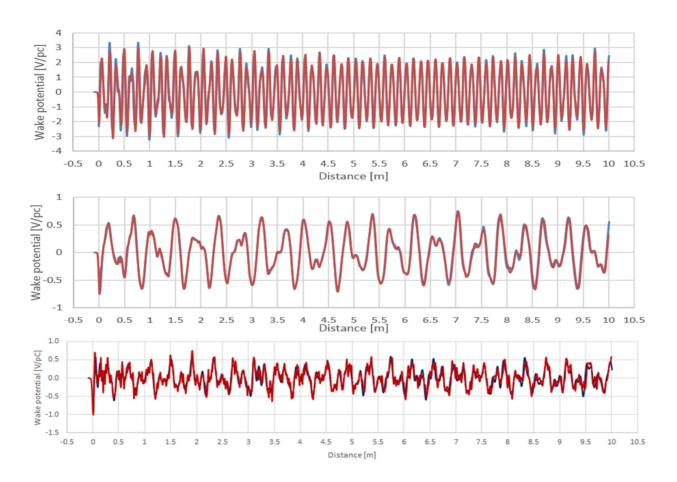
Figure 2: Single bunch wake potential in 10m for a) 2.1 GHz warm cavity (top); b) 704 MHz warm cavity (middle); c) 704 MHz booster SRF cavity (bottom). Blue curves are from the reconstruction of Eigen mode simulation, and red curves are from CST Particle Studio<sup>TM</sup>.
