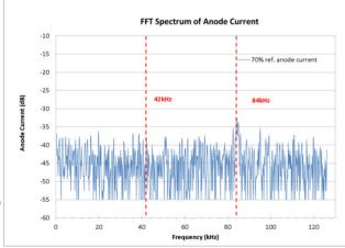
Figure 8: FFT spectrum measured directly by TDS2014B scope from magnetron power supply anode current monitor.
