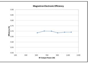
Figure 5: Electronic efficiency in operation parameter range.
