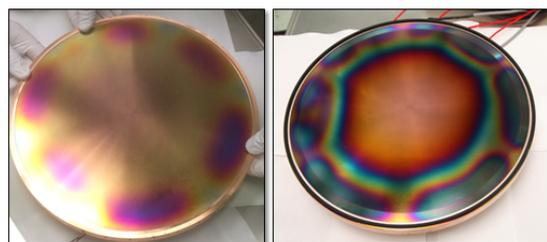
Figure 3: Interior surface of endplates. The variation in coloring is due to difference in TiN coating thickness.
