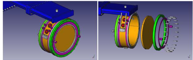
Figure 1: 3D model (left) and exploded view (right) of modular cavity.
