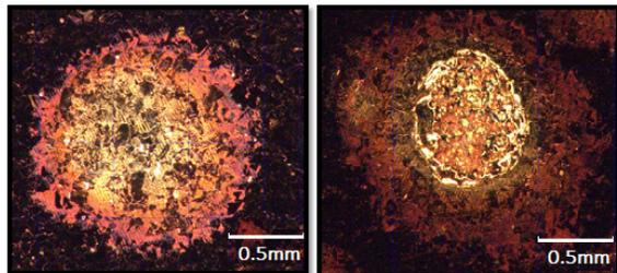
Figure 5: Microscopic images of typical breakdown “pits” with and without melted core present.
