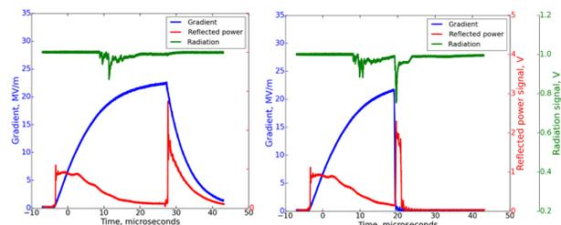
Figure 2: Envelope of pickup signal (blue), NaI radiation detector (green), reflected power (red) for normal event (left) and breakdown event (right).
