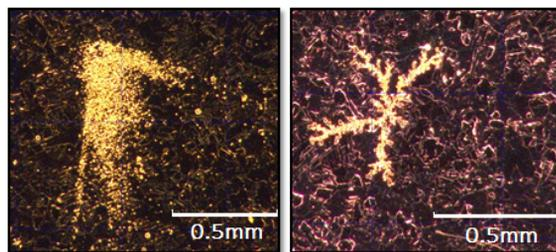
Figure 4: Typical cavity damage observed after high-power  $B=0\text{T}$  run.
