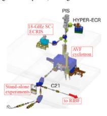
Figure 1: RIBF injector complex including the 18 GHz SC-ECRIS.
