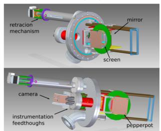
Figure 3: Emittance meter design details.
