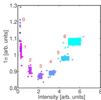
Figure 6: The bunch-by-bunch beam size ( $1\sigma$ ) measurement in the  $7 \times 12$  buckets for an LHC beams in the PS at extraction energy.
