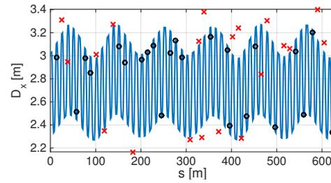
Figure 3: Comparison between measured (markers) and simulated dispersion (solid line). The red markers represent values in disagreement with the model.
