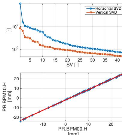
Figure 1: Singular values of the dispersive orbits in the horizontal and vertical planes (top). An example of correlation between two PUs (bottom). From the two plots we can conclude that the  $D_x$  within the  $\frac{\Delta p}{p}$  region explored during the radial scan.
