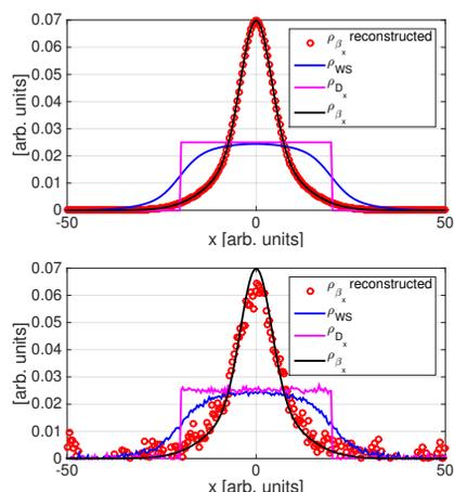
Figure 4: Deconvolution without noise in the measured signal,  $\lambda = 0$  (above). Simulating the effect of noise,  $\lambda = 0.003$  (below).
