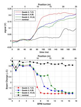
Figure 2: BLM signals (top) and BPM intensity measurements (bottom).
