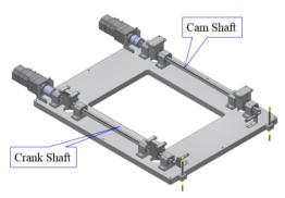
Figure 7: Sub assembly of XM.
