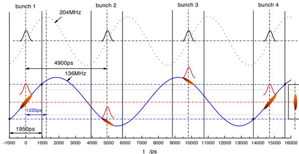
Figure 5: The unit time sequence of synchronous sweep under two thirds RF frequency.
