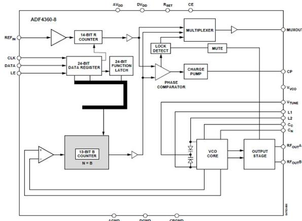
Figure 6: Function block diagram of ADF4360-8.
