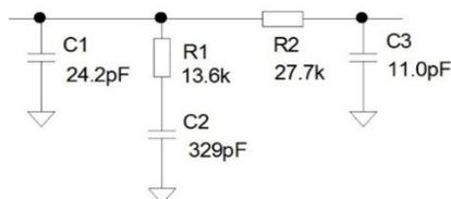
Figure 7: The loop filter.
