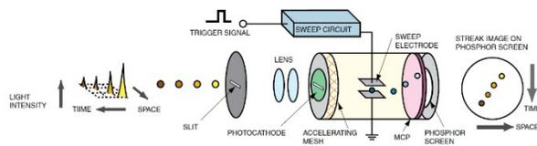
Figure 1: Operating principle of the streak camera.
