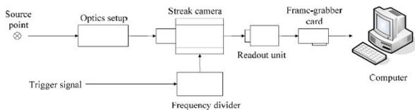
Figure 3: The system configuration of streak camera.
