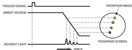
Figure 2: Operating timing (at time of sweep).
