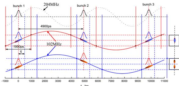
Figure 4: The unit time sequence of synchronous sweep under half RF frequency.
