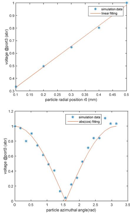
Figure 4: The voltage 3 FFT value versus particle radial position  $r_0$  (top) and voltage 3 FFT value versus particle azimuthal angle  $\theta_0$  (bottom).
