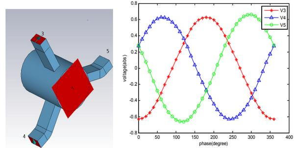
Figure 2. Simulation model in CST (left). The voltage achieved at port 3~5 (right).
