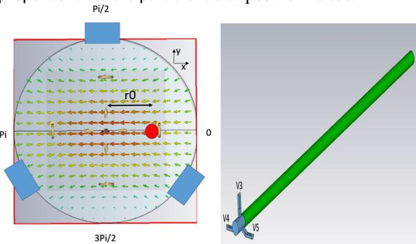
Figure 3. The field map in the metal tube behind dielectric-lined waveguide (left). The model of 200 mm dielectric-lined waveguide with BPM (right).
