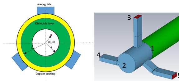
Figure 1. Cross section view of the dielectric accelerating structure (left). BPM coupler model in CST Microwave Studio (right).
