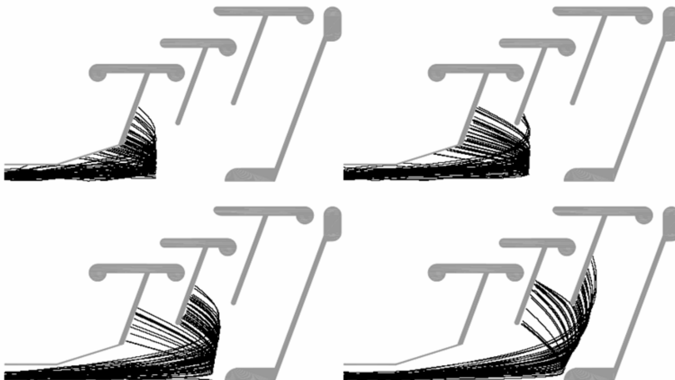
Figure 5-16: 50 Sample trajectories for 50, 125, 200 and 275 keV electrons. The electrons with the highest energies are collected on the electrodes with the lowest potential.
