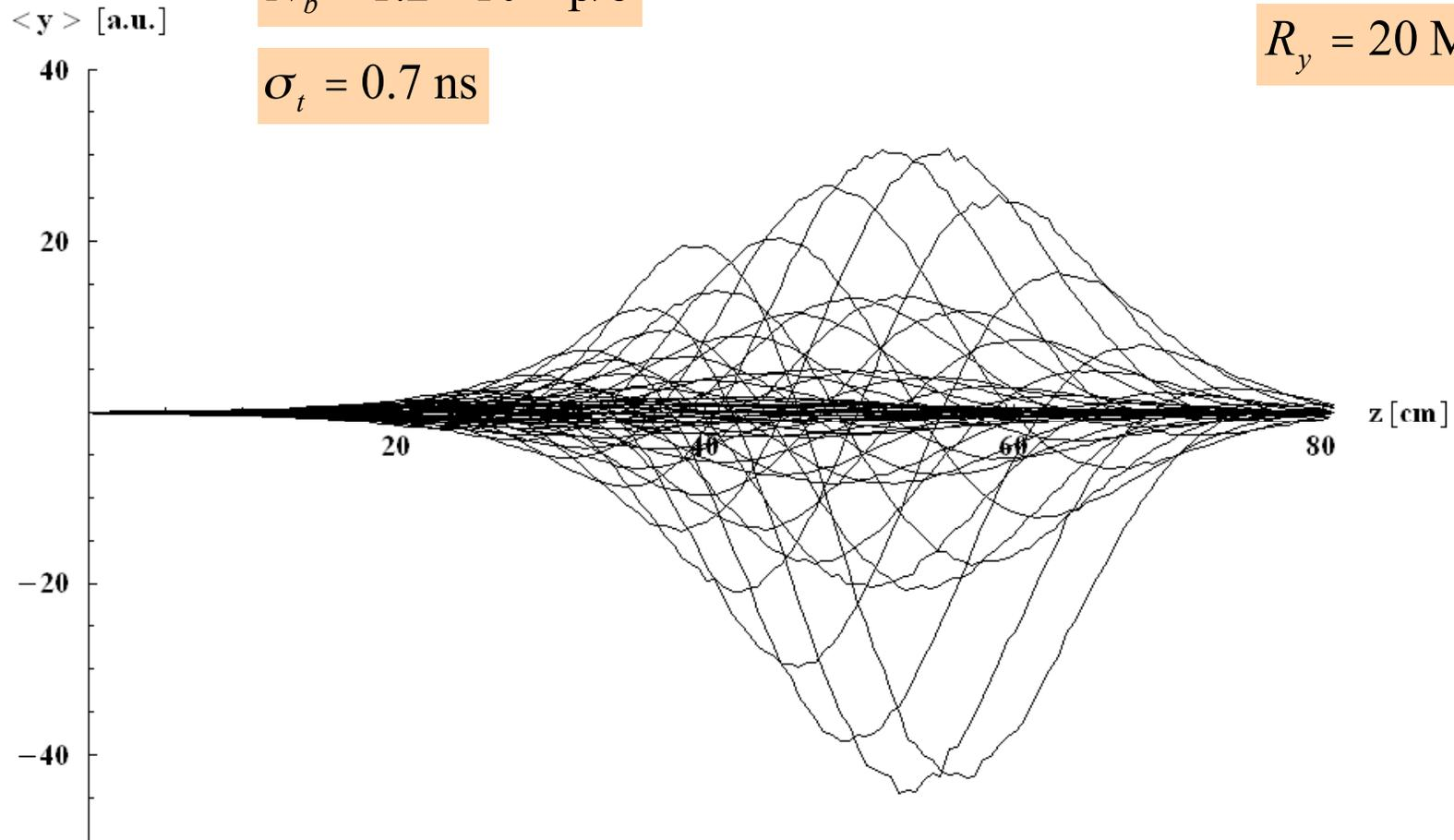
SPS TMCI simulated with HEADTAIL using a BB-impedance
