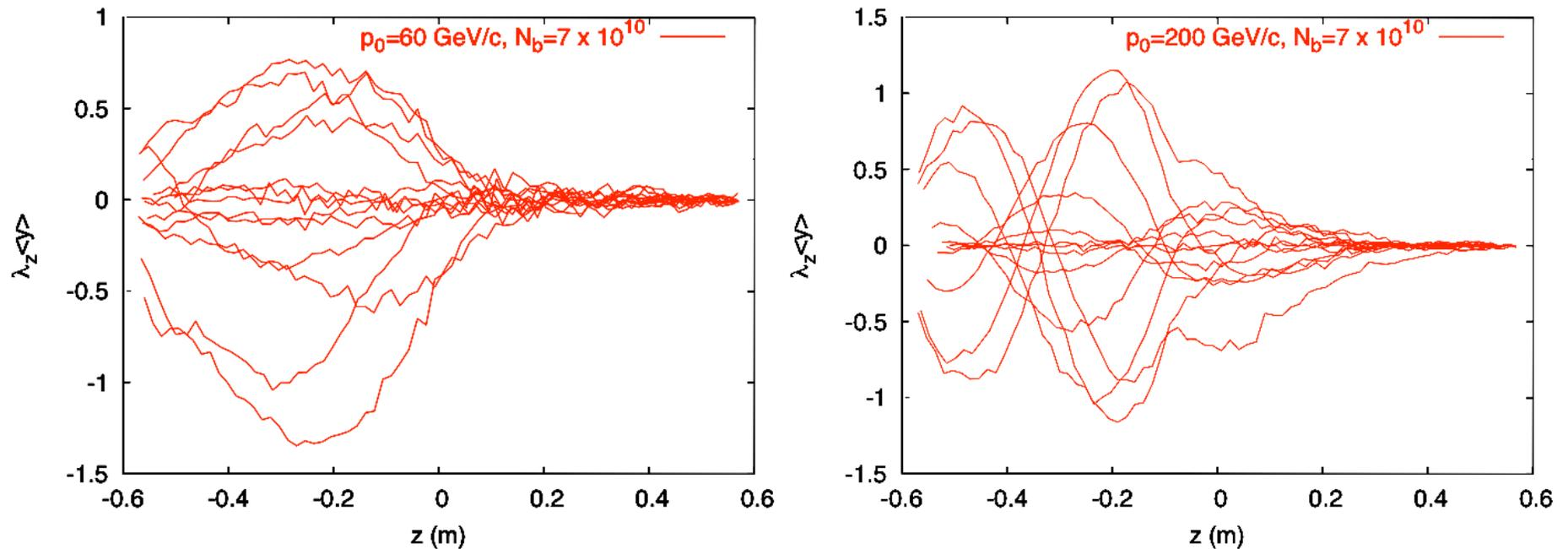
The **coherent motion** appears along the bunch with a **typical TMCI pattern**.
