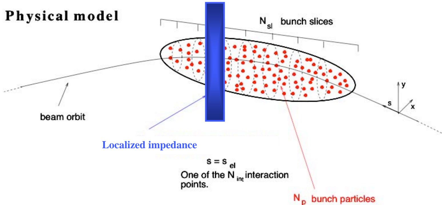
Simulation model: electron cloud and bunch are both modelled as ensembles of macro-particles (typically 100000) and the bunch is divided into an adjustable number of slices (typically 50).
