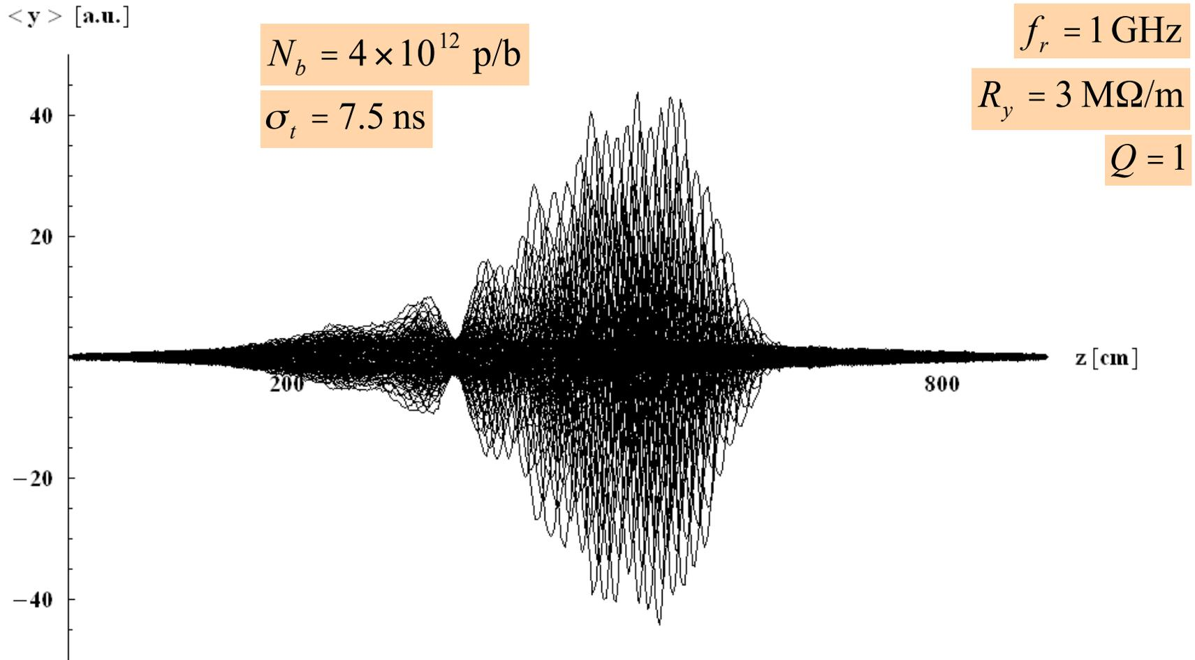
PS TMCI simulated with HEADTAIL using a BB-impedance
