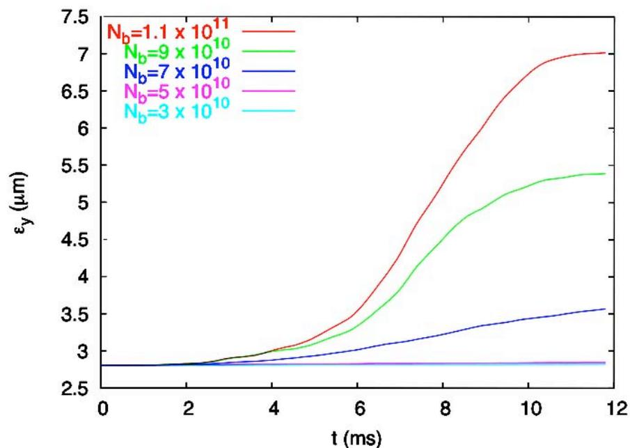
Example at 40 GeV/c with centroid motion and emittance evolution at different bunch intensities:
