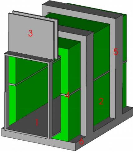
Figure 1: Schematic view of the SNS kicker where it is possible to observe the busbar (1), the ferrite (2), the end-plates of the busbar (3), the strips (4), a frame (5) and a base (6).
