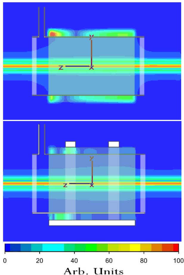
Figure 4: Vertical cutting plane at  $x=0$  of the kicker magnet without (upper panel) and with (lower panel) the metallic frame showing contour plot of  $|B_x|$  for  $f = 35$  MHz.
