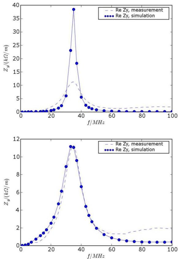
Figure 3:  $Z_y$  vs. frequency for the case  $Z_{ext} = \infty$ . The dotted line follows from simulation and dashed line from experimental measurements[4, 5].
