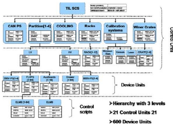
**Figure 2: TILECAL FSM Architecture**
