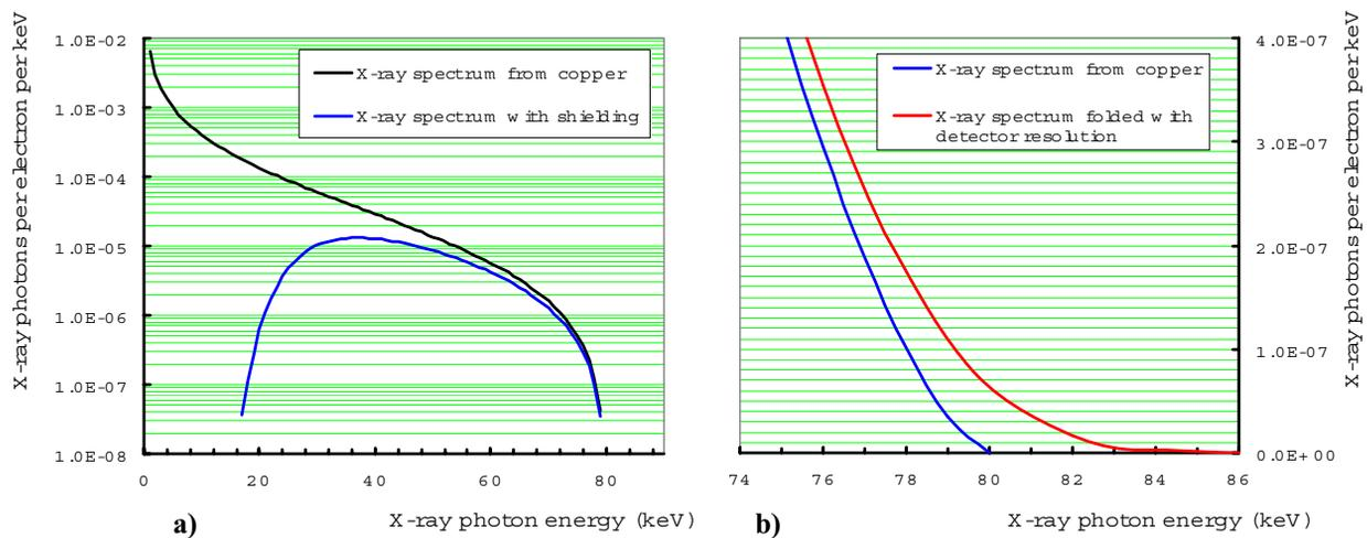
Fig. 2 a) Calculated x-ray spectrum for a DEE potential of 80 kV and the spectrum attenuated with 0.5 mm copper and 2 mm aluminium. b) Calculated x-ray spectrum after convolution with detector resolution.
