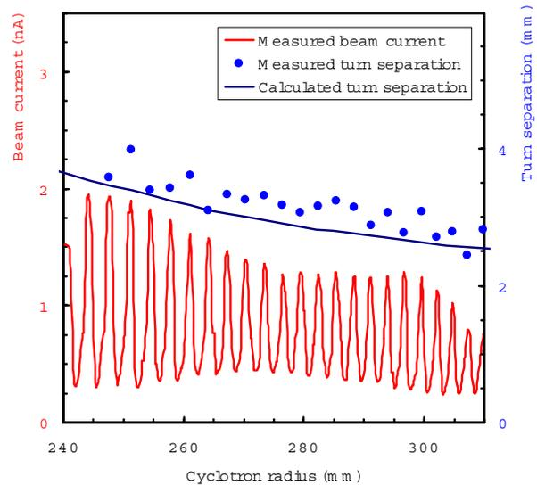
Fig. 5. Beam current trace showing individual turns at 120 kW RF power. The measured turn separation is in good agreement with the calculated turn separation.
