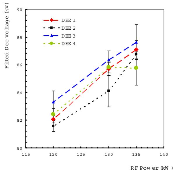
Fig. 4. Final set of DEE voltage measurements at different RF power levels showing a DEE potential spread of  $\sim 2$  kV.
