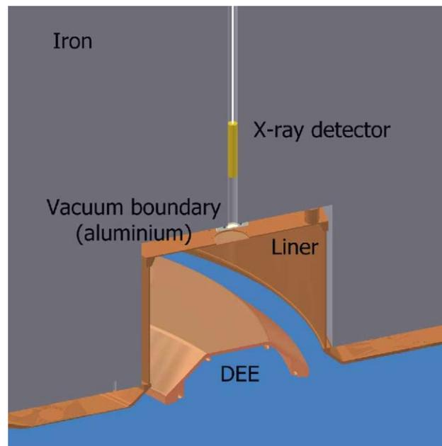
Fig. 1. Cross sectional view of the X-ray detector mounted behind the liner.
