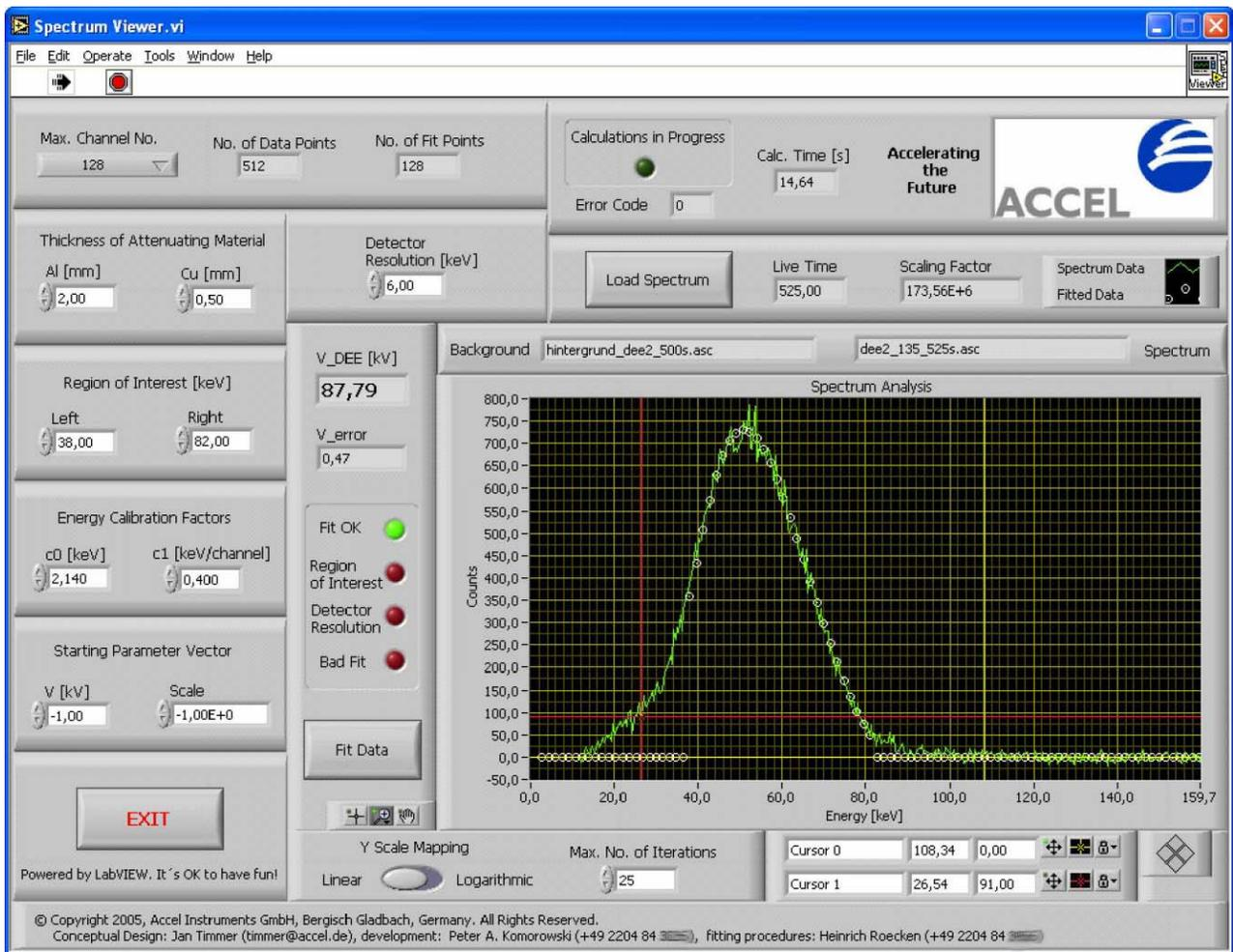
Fig. 3. PicoSpec Gold Spectrum Viewer. The measured spectrum is shown in green, the fitted spectrum (87.79 kV) is plotted with white circles.
